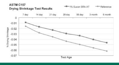
Cement content - 517 lbs/yd $^3$  (307 kg/m $^3$ ) W/C = 0.50 Air Content = 7.4% Slump = 5  $^1$ /4" (130 mm)
